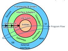
Entities: Entities encapsulate enterprise-wide business rules. An entity can be an object with methods, or it can be a set of data structures and functions
